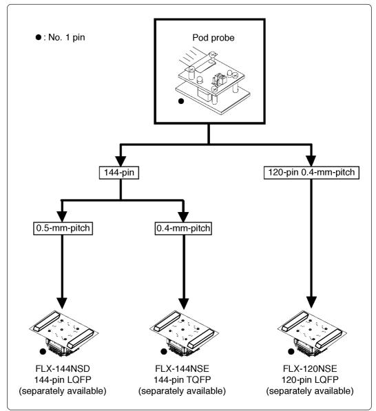
Figure 3.5 Connecting the target system
